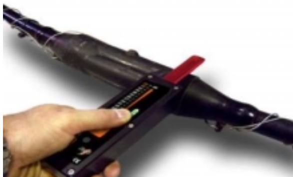
Detecting a PD source with the capacitive sensor
