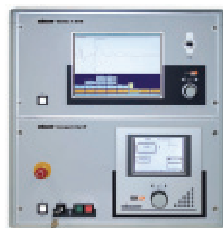
Test van installation with 19" rack containing SPG 40 Control Panel and T 30 M
