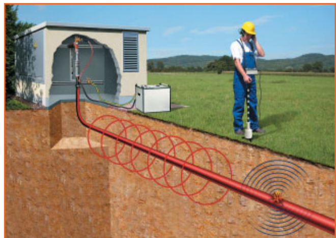
Fault location with SWG and Digiphone
